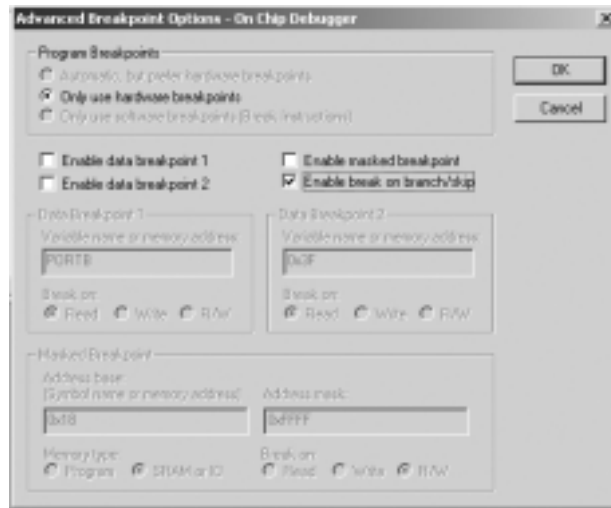
Figure 3-6. Enable Break on Branch/Skip
