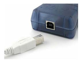
When the AVRISP mkII is connected to the PC, and if the USB driver is installed, the green LED inside the AVRISP mkII close to the USB connector will be lit. The main status LED will be red before target is detected.
